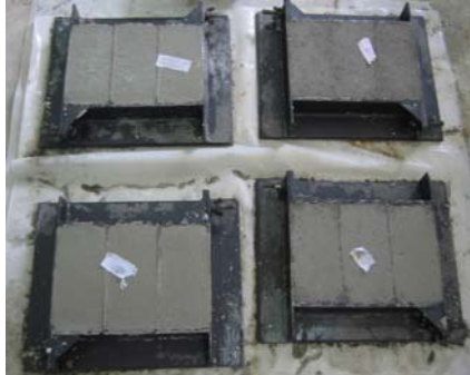
Figure 2: Fabrication of concrete paving block specimens
