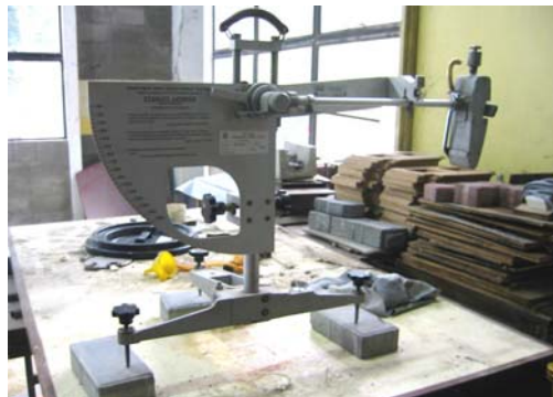
Figure 4: Skid resistance test
