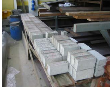
Figure 3: Air curing of paving block specimens concrete
