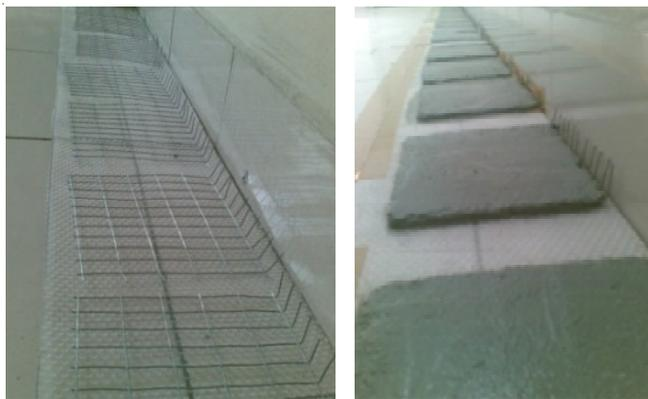
Fig. 2. (a) galvanized mesh before filling with concrete (b) nano-TiO<sub>2</sub> concrete mixed Panels
