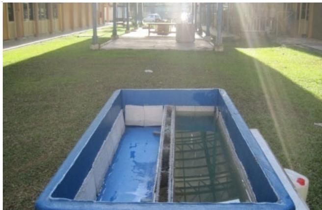
Fig. 1. 1:20 Scale model of designed pond with nano-TiO<sub>2</sub> concrete sheets under the sunlight
