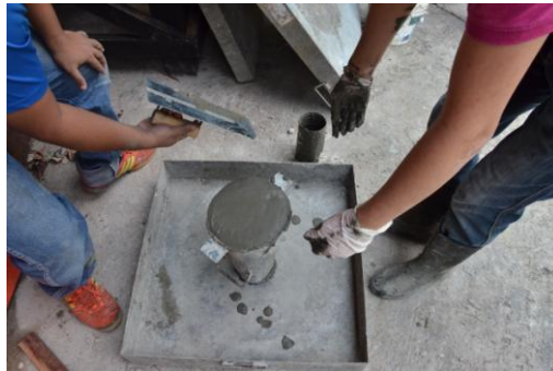
Figure 4: Inverted slump test for lightweight foamed concrete
