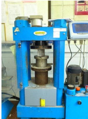
Figure 5: Compressive strength test setup
