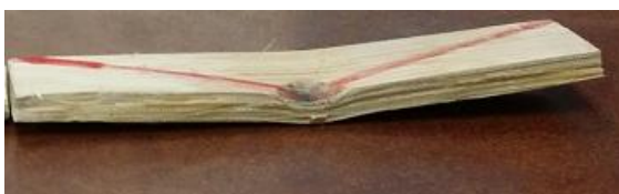
Figure 9: Half part of the specimen after second impact
