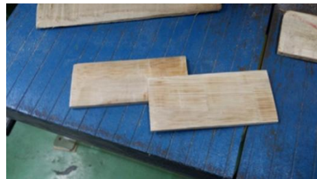
Figure 2: Flat plate specimen of pure bamboo
