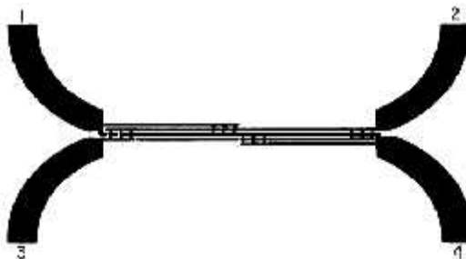
Figure 1.3 Interdigitated 3-dB Coupler (Lange et al. , 1969)
