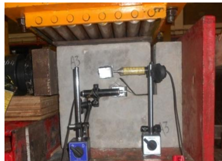
(b) Location of the LVDTs
