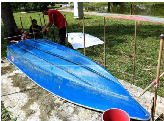
Figure 5. Contact method measurement using strings and rules.
