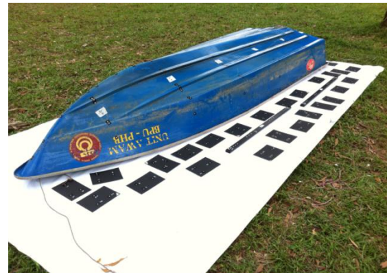
Figure 3. Retro reflective targets installed on the boats.
