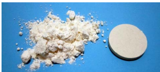
Fig. 2 Ground rice samples were pressed into pellets before LIBS analyses
