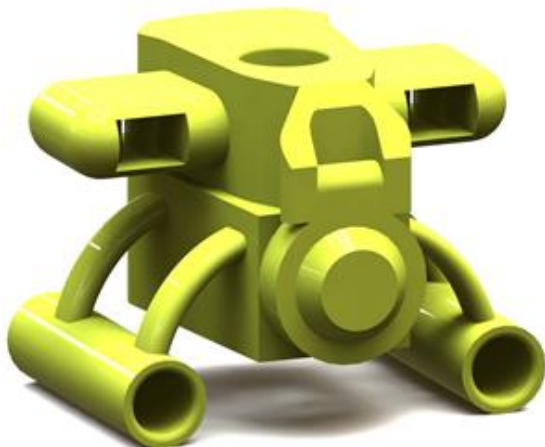
Figure 4. Concept design of ROV based on combination of 'WorkClass and 'EyeBall' types
