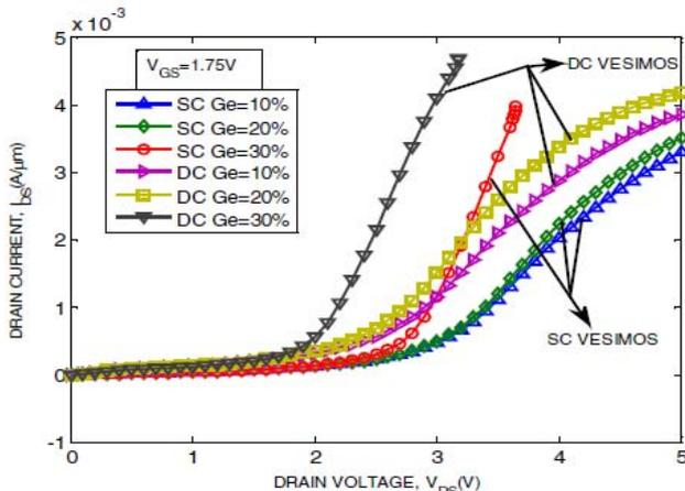
Fig. 6. Comparison of output characteristics,  $I_D$ - $V_D$  of variation Ge mole fraction for Single Channel and Double Channel VESIMOS
