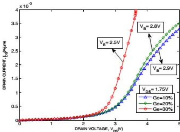
Fig. 5. Output Characteristics,  $I_D$ - $V_D$  of variation Ge mole fraction for Single Channel VESIMOS
