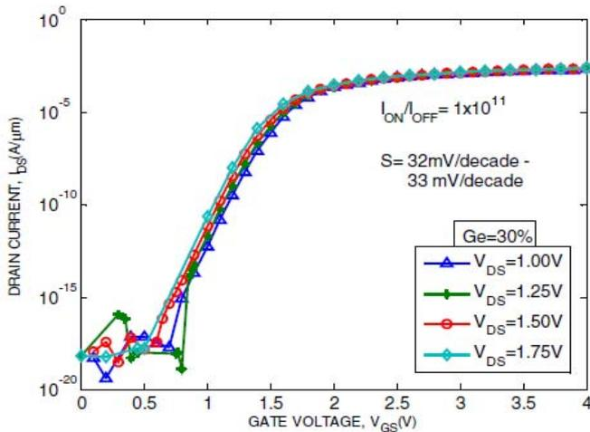
Fig. 2. Transfer Characteristics,  $I_D$ - $V_G$  of VESIMOS for  $Si_{0.7}Ge_{0.3}$
