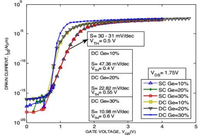
Fig. 3. Comparison of transfer characteristics,  $I_D$ - $V_G$  of variation Ge mole fraction for SC and DC VESIMOS at  $V_{DS}=1.75V$
