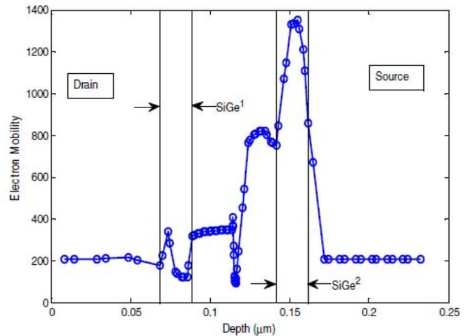
Fig. 7. Electron mobility versus depth of double SiGe VESIMOS for  $V_{DS}=1.75V$
