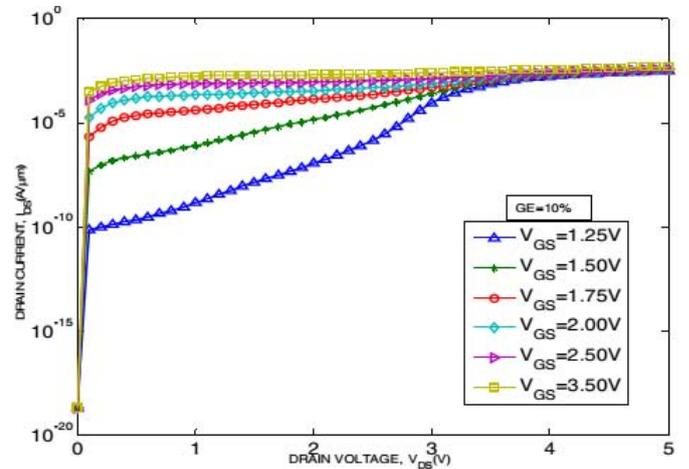
Fig. 4. Output Characteristics,  $I_D$ - $V_D$  of VESIMOS for  $Si_{0.9}Ge_{0.1}$  at different  $V_{GS}$
