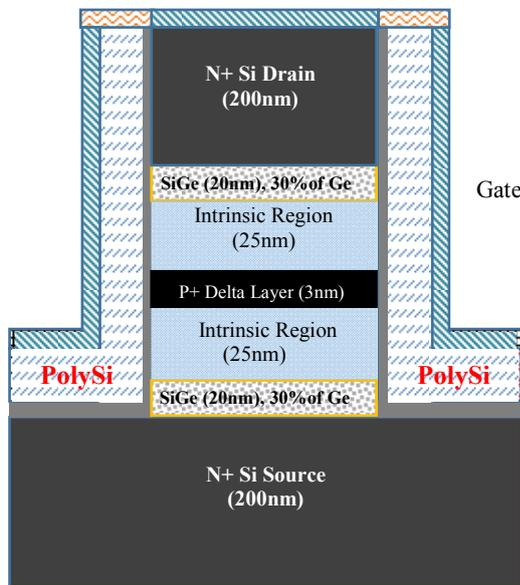
Fig. 1. Double layer SiGe VESIMOS device structure with dimension of  $L=93\text{nm}$ ,  $d=200\text{nm}$ , respective thickness of source, intrinsic region, P+ delta layer, SiGe layer, drain and both layer fraction of Ge is 30%.
