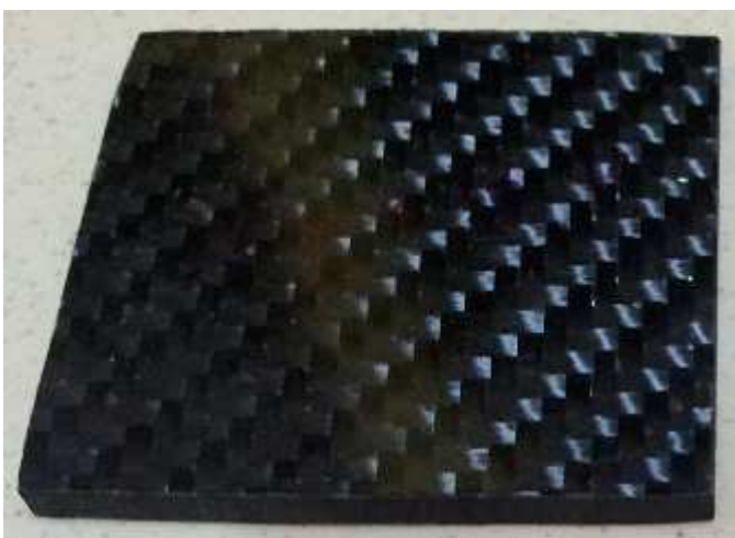
Figure 1. CFRP work-piece material
