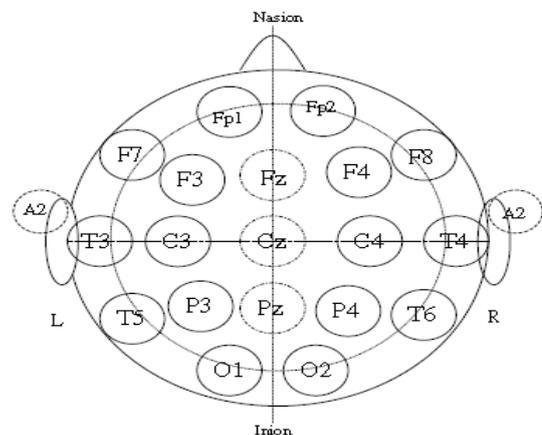
Fig. 1. Electrode placement 10-20 international system [12]
