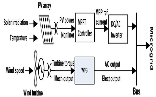
Fig. 1. Block diagram of PV/Wind hybrid system
