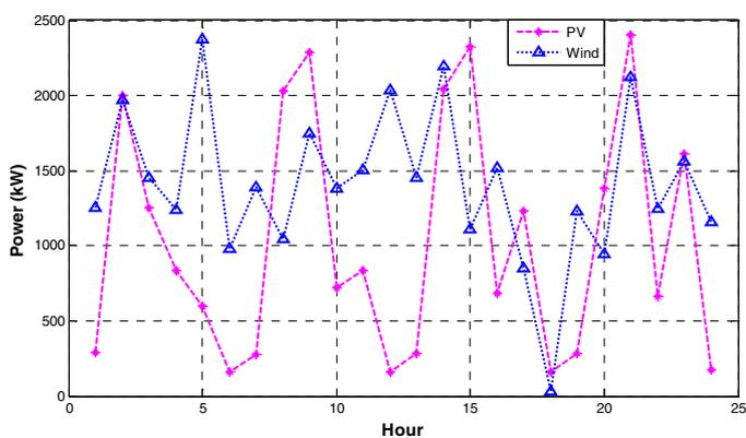
Fig. 4. PV and wind power outputs throughout the day
