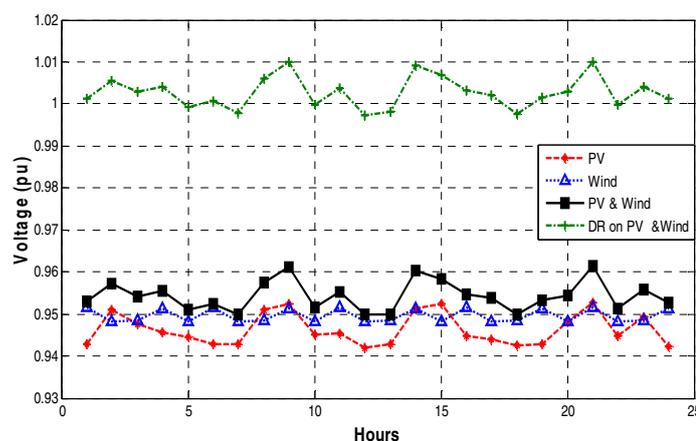
Fig. 7. Effect of demand response at bus 14 on system hourly voltage profile
