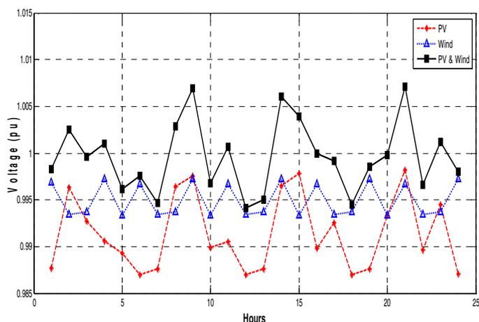
Fig. 3. Hourly voltages at bus 14 due to PV, wind and hybrid PV/wind
