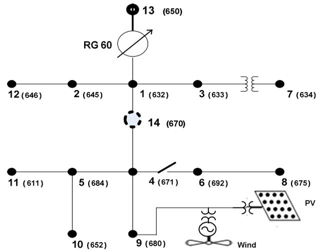
Fig. 2. Autonomous MG bus feeder
