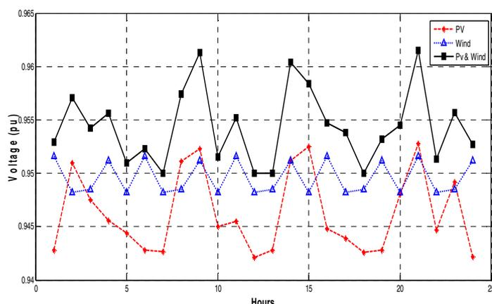
Fig. 6. Hourly voltage variations at bus 14 due to 45% load increase
