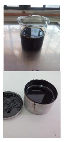
Figure 1 Bio-oil sample and standard bitumen
