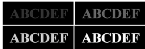
Figure 5 Image with Various TBSI. Top left: TBSI = 0.8039 ; Top right: TBSI = 0.6078 , Bottom left: TBSI = 0.2157 ; Bottom right: TBSI = 0.0157
