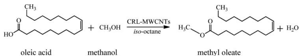
Figure 5. Esterification reaction of oleic acid and methanol catalysed by the CRL-MWCNTs.
