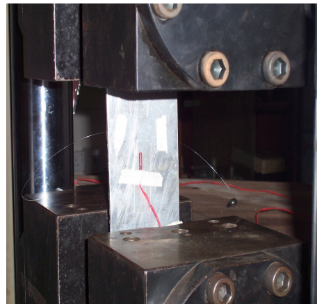
Fig. 5a: Fiber optic sensor and foil gauge bonded to aluminum specimen (b) load instron machine for tensile testing
