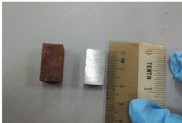
Figure 3. Carbon steel coupon before and after polishing.
