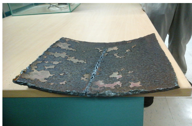
Figure 2. Carbon steel oil and gas pipeline grade API 5L-X70.
