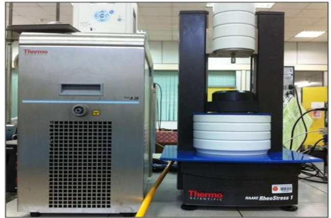
Figure 1 Thermo Scientific Haake Rheo Stress 1 Dynamic Shear Rheometer
