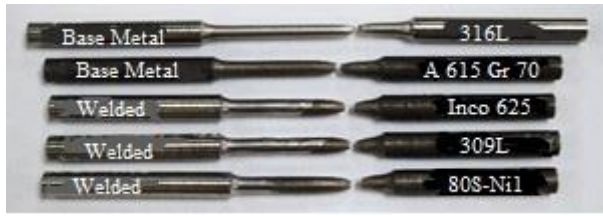
Figure 4 Photograph of fractured tensile specimens of the base metal and welded specimens
