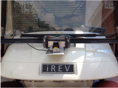
FIGURE 6: Hokuyo LRF placed on iREV.
