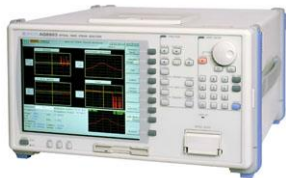
Brillouin Optical Time Domain Reflectometry (BOTDR) for concrete structure health monitoring
