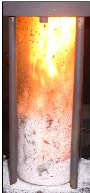
Plate 4.1-7: Suspension burning of rice husk at fluidising velocity of 5 U_{mf} (sand size 595 – 841 \mu\text{m} )
