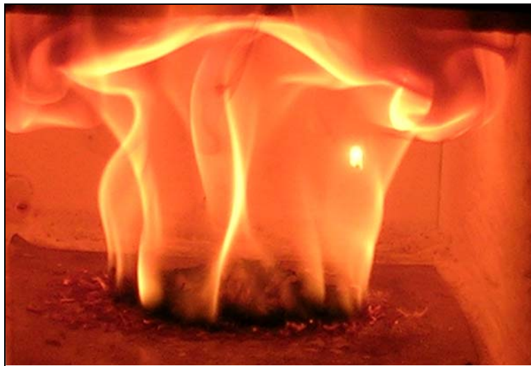
Plate 4.1-2: Higher flaming times for a group of rice husk particles spread widely apart in the muffle furnace (650 – 750°C)
