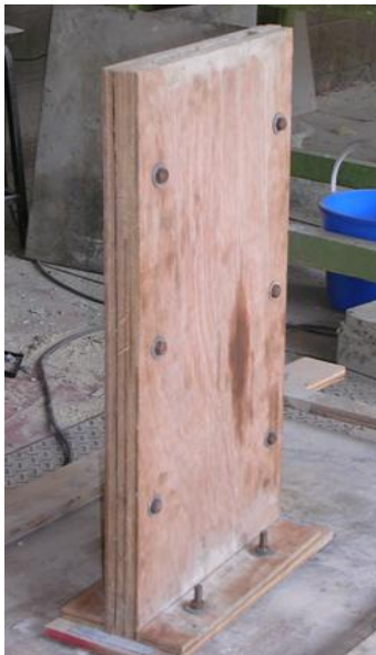
Figure 3.10: Mould used to cast thin FC elements
