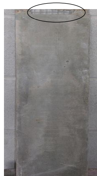
Figure 3.12: FC element showing wire mesh inside
