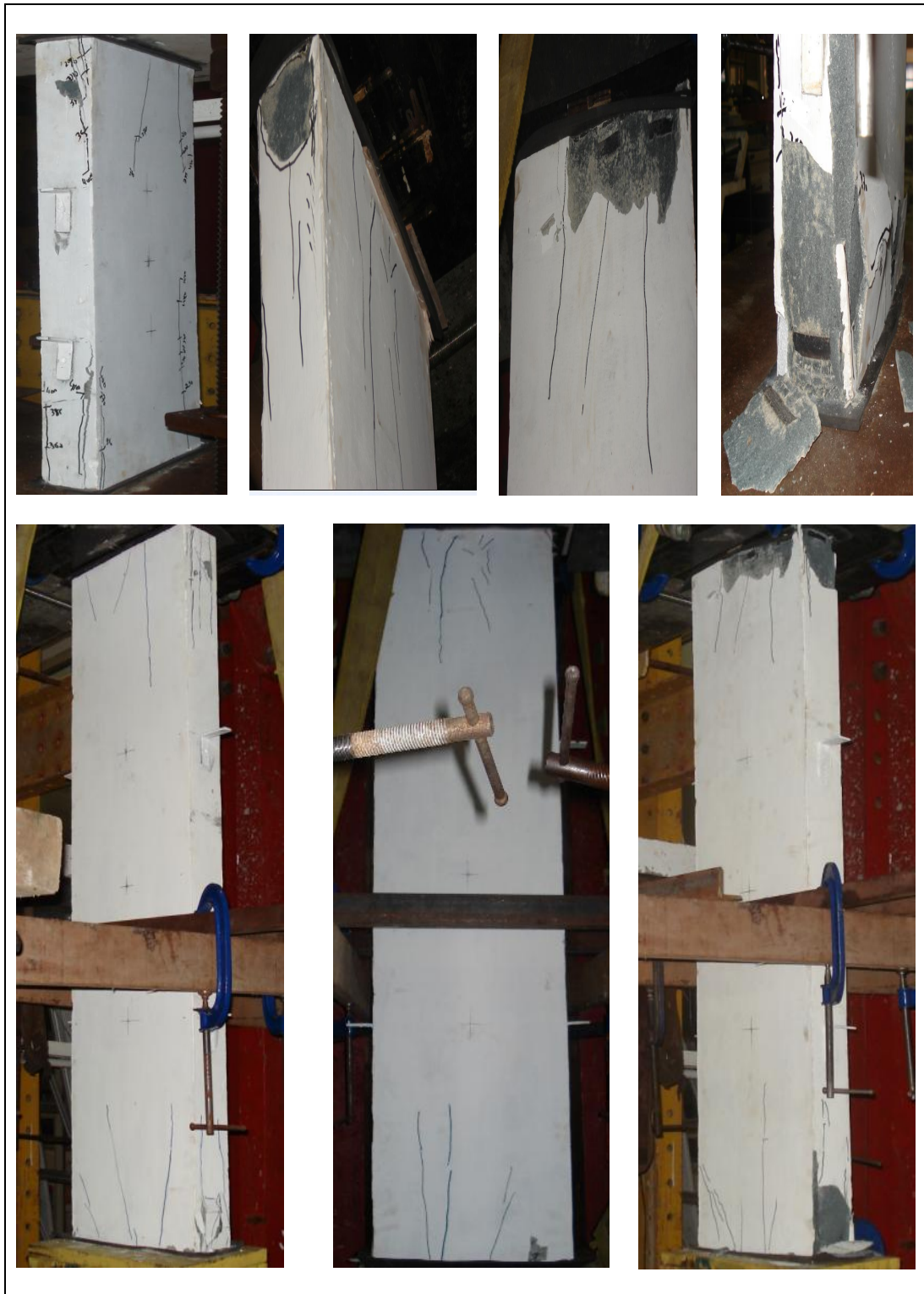
Figure 5.29: Failure mode of sandwich wall elements with reinforcement (wire mesh and others) in compression
