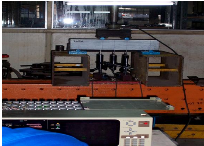
Figure 3.28: Test setup for prism beams under flexure (bending)
