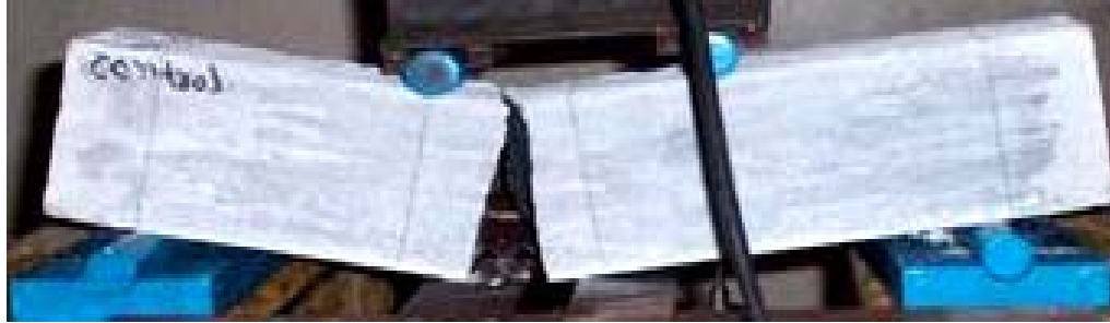
Figure 5.13: Failure mode of control prism beam in flexure
