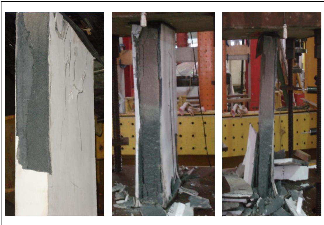
Figure 5.28: Failure mode of sandwich wall elements without wire mesh in compression
