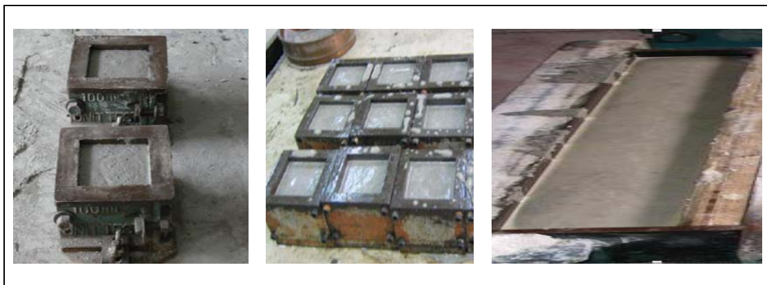
Figure 3.15: AC filled in moulds up to 80%.
