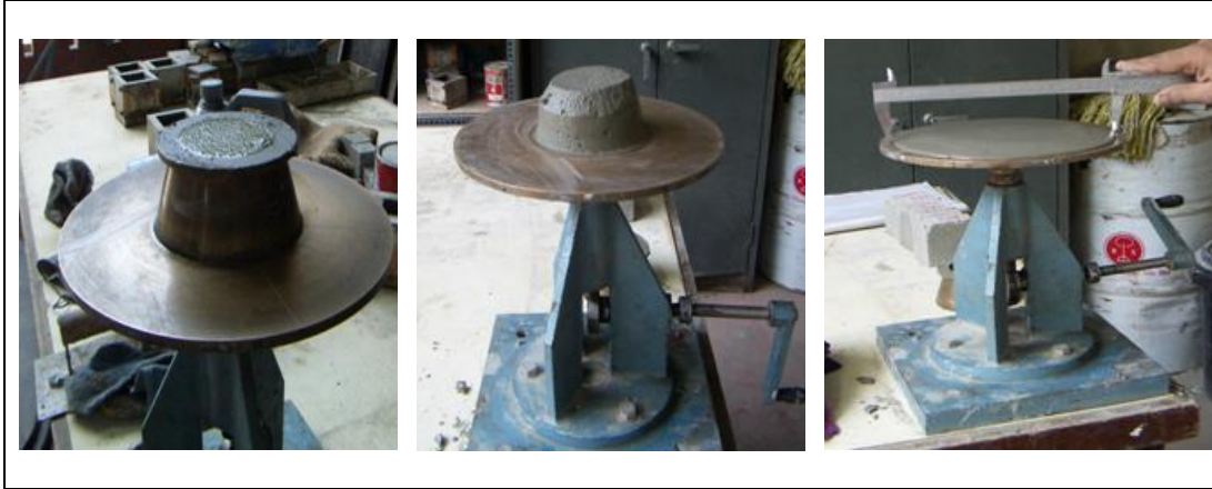
Figure 3.23: Flow table test
