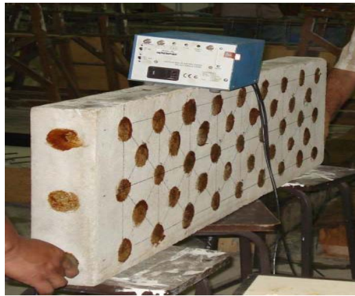
Figure 3.32: A pictorial view of UPV test in progress
