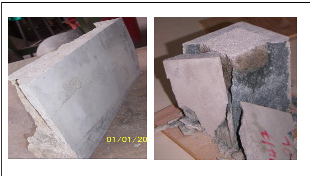
Figure 5.11: Failure mode of sandwich specimens without mesh in compression
