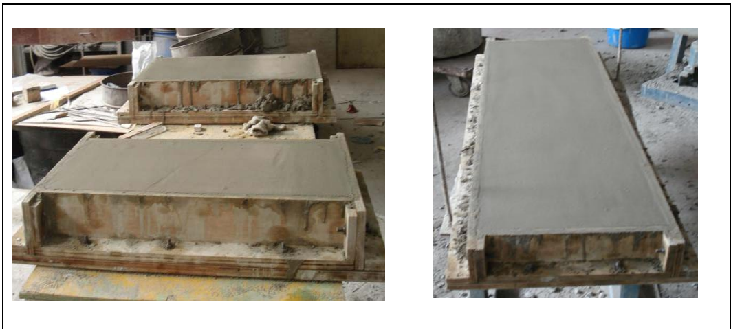
Figure 3.21: Sandwich specimens after casting of encasement
