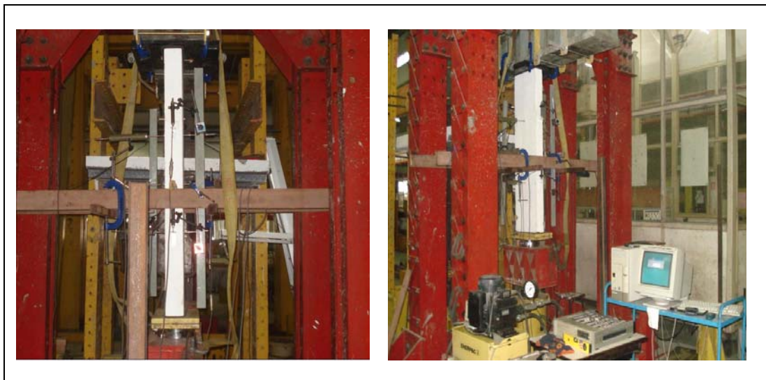
Figure 3.27: Test setup-II for wall panels under compression.
