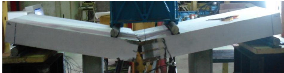
Figure 5.36: Failure mode of sandwich wall element without wire mesh in flexure
