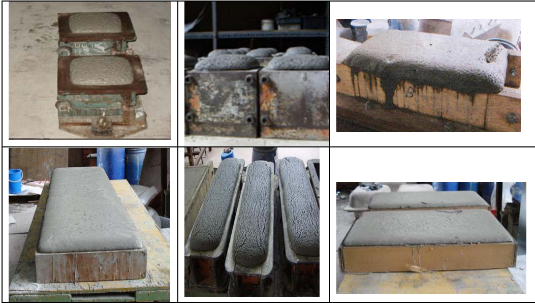
Figure 3.16: AC specimens after expansion
