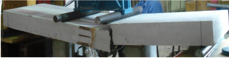
Figure 5.35: Failure mode of control wall element in flexure
