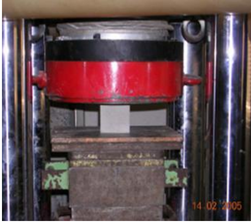
Figure 3.24: Test setup for cubes.
