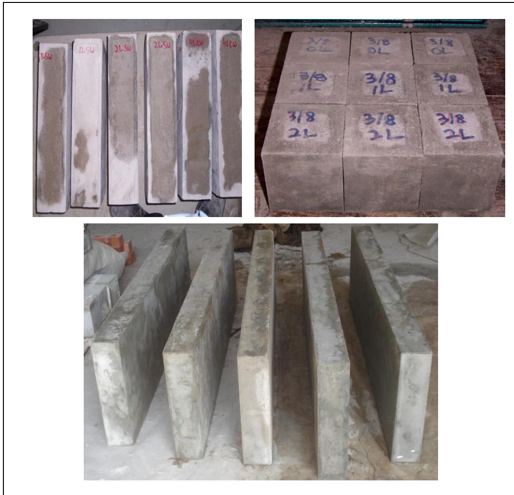
Figure 3.22: Sandwich specimens under curing process
