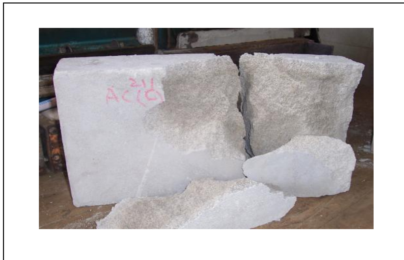
Figure 5.10: Failure mode of control specimen in compression
