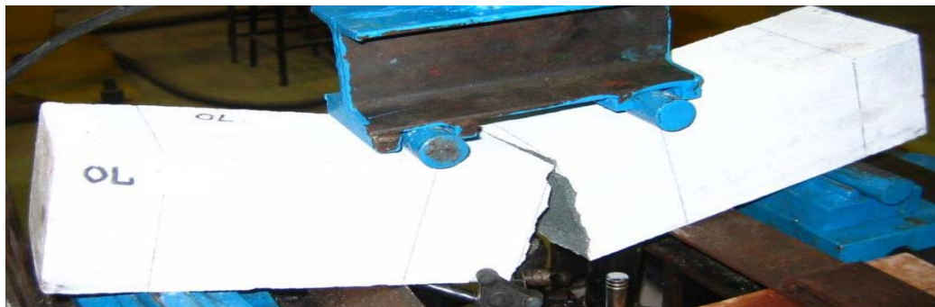
Figure 5.14: Failure mode of sandwich prism beam without wire mesh in flexure
