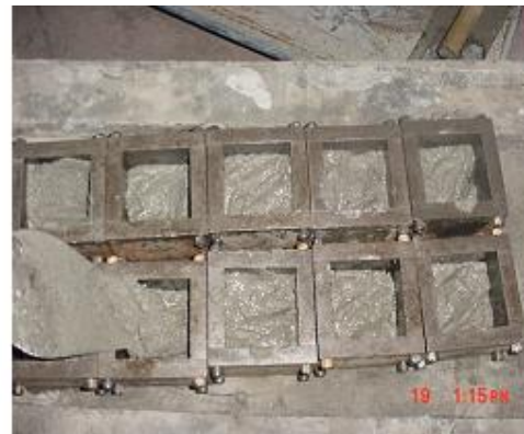
Figure 3.10: Casting into moulds size 70.6x70.6x70.6 mms
