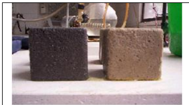
Figure 5.18: Effect on MBC (left) and control (right) mortar subjected to acid attack after 600hours of immersion
