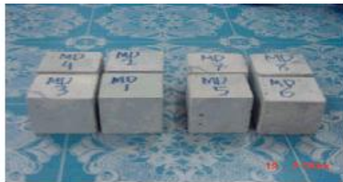
Figure 3.15: 50x50x50mm cubes cut from 100x100x100mm by cutter machine
