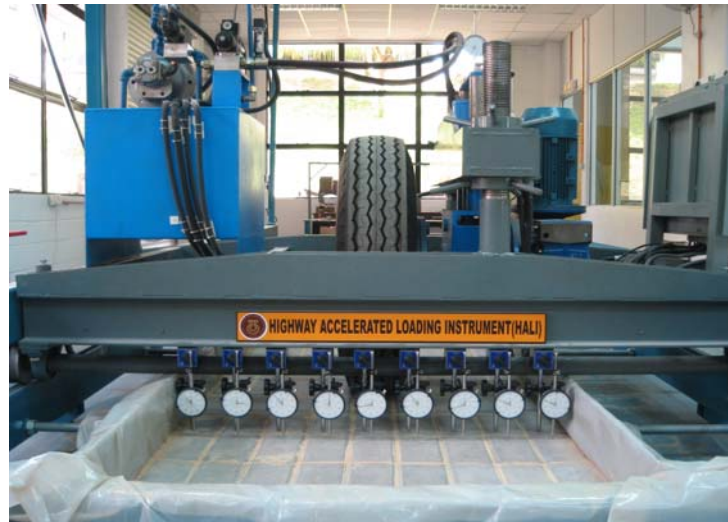
Figure 3.20 Measurement of pavement model deformation using the dial gauges
