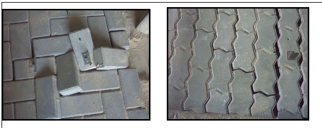
Figure 3.10 CBP failure after testing
