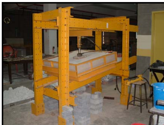
Figure 3.18 Push in test on sloping section
