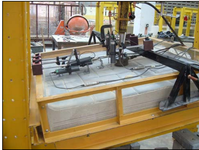
Figure 5.10 Measurement horizontal creep on push-in test
