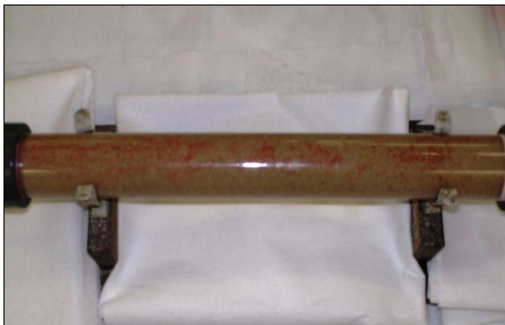
Figure 4.53 The sand pack after waterflooding succeeded by surfactant polymer injection
