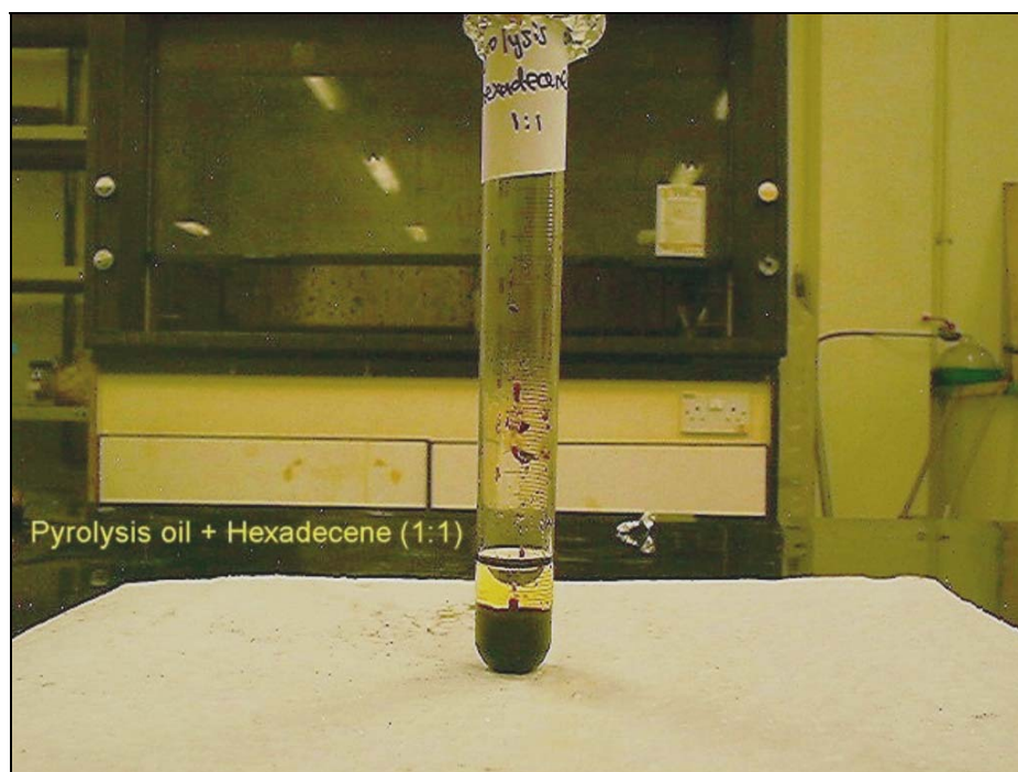
Figure 4.2 The dissolubility of pyrolysis oil in hexadecene in 1:1 volume fraction
