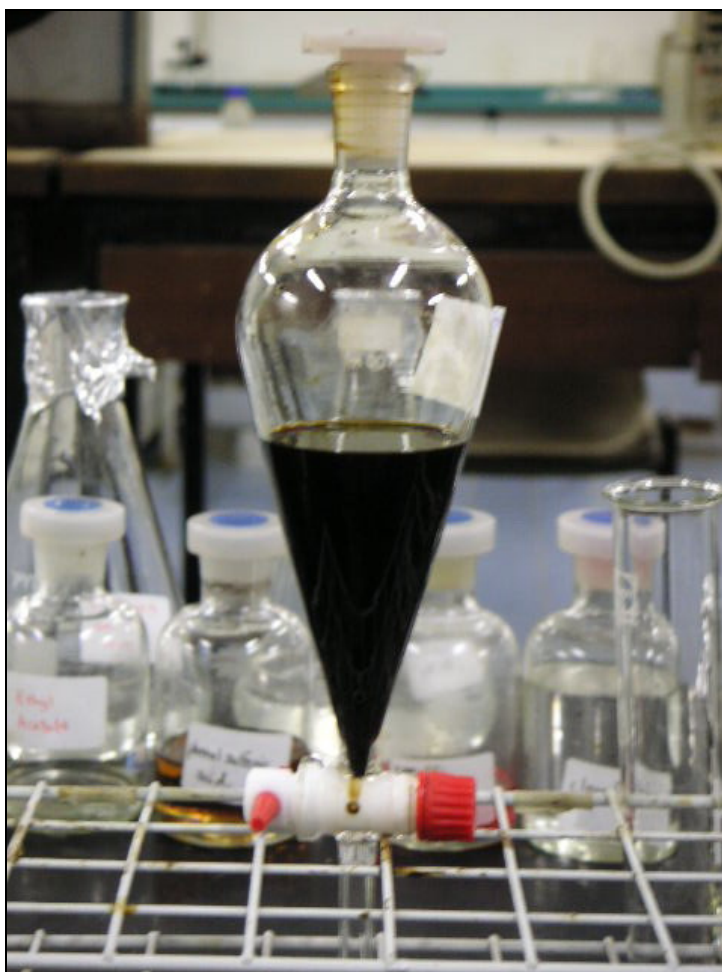
Figure 3.8 Extraction of phenol from pyrolysis oil
