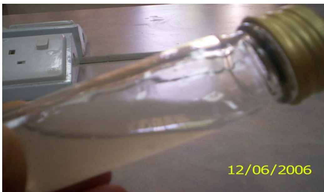
Figure 4.40 Gelling of refined xanthan gum after 5 days at 60° C
