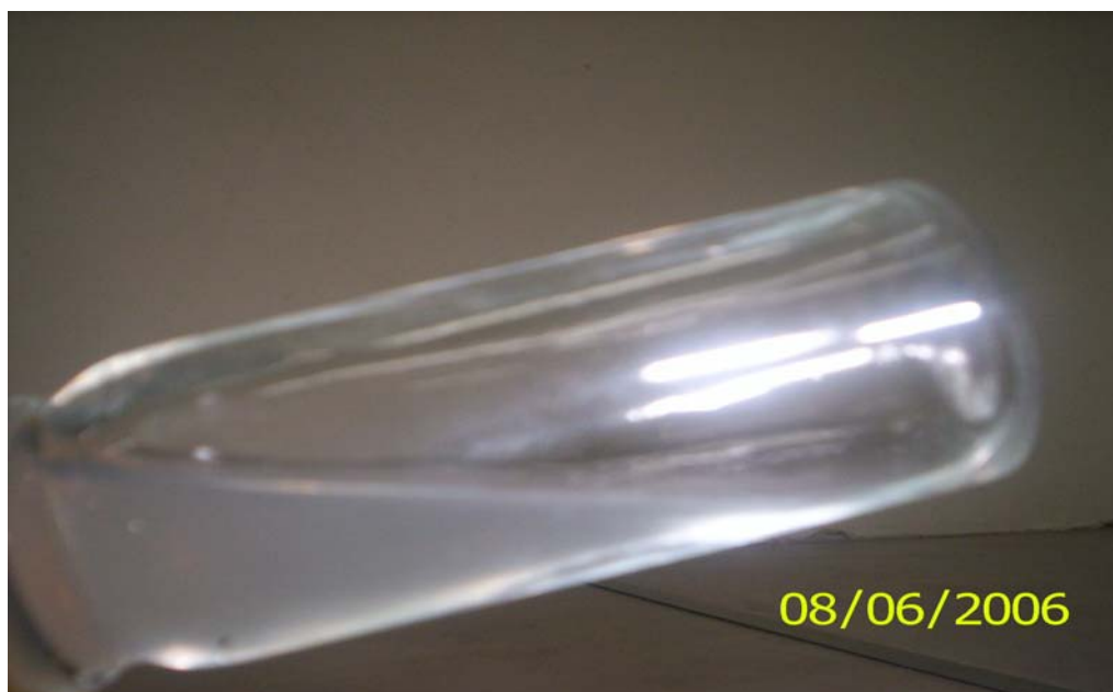
Figure 4.24 Gelling of refined xanthan gum after 2 days at 60° C
