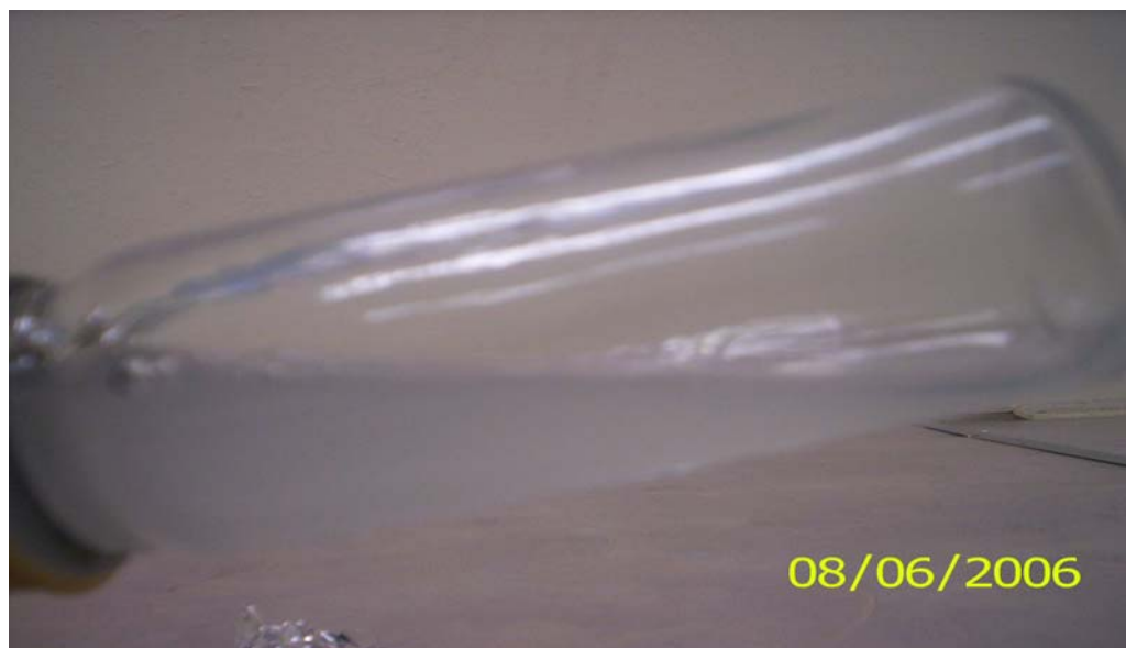
Figure 4.39 Gelling of refined xanthan gum after 2 days at 60° C
