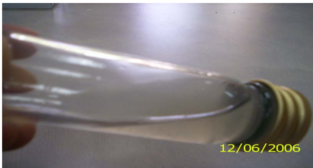
Figure 4.25 Gelling of refined xanthan gum after 6 days at 60° C
