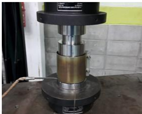
Figure 2 Die set covered with steel coil heater
