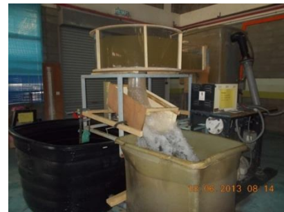
Figure 2 Vortex pool system model constructed in Universiti Teknologi Malaysia (UTM)
