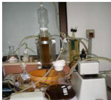
Figure 2 H 2 gas fermentation by using Sweet sorghum and Enterobacter aerogenes ADH-43 in a packed-bed reactor continuous system
