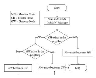
Figure 2 Describes new node joining in CNet(G)
