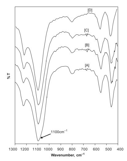
**Figure 2** IR spectra for synthesis zeolites: [A] 30 SiO<sub>2</sub>/Al<sub>2</sub>O<sub>3</sub>, [B] 30 SiO<sub>2</sub>/Al<sub>2</sub>O<sub>3</sub>, [C] 70 SiO<sub>2</sub>/Al<sub>2</sub>O<sub>3</sub>, [D] commercial HZSM-5
