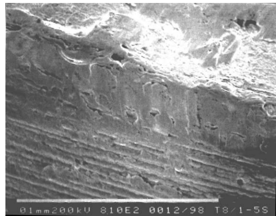
Fig. 5. An SEM image of Tool A after cutting for 5 s, showing galling and pitting on the rake and flank faces (at 25 m/min and 0.14 mm per tooth).
