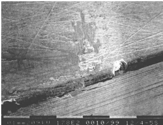
Fig. 7. Galling and pitting on the rake face of Tool C after cutting for 5 s. Adhesion of relatively large chip particles at the cutting edge was also observed (at 50 m/min and 0.14 mm per tooth).
