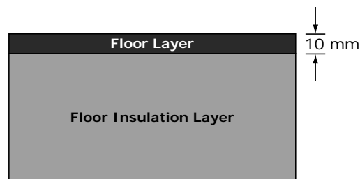
Figure 8: Floor Setup Scheme
