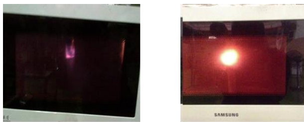
Figure 5(a) MW gasification without AC Figure 5(b) Plasma gasification with AC
