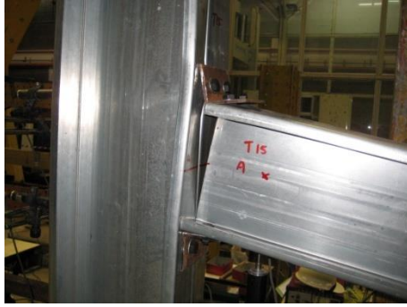
Figure 7 Failure mode for 6 mm thickness of flange cleat which is column flange in bending
