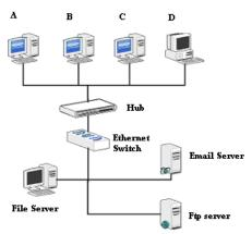
Figure 2 Ethernet communications through Hub.
