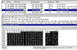
Figure 5 Encrypted Data Payload with Secure Socket Layer (SSLv3).
