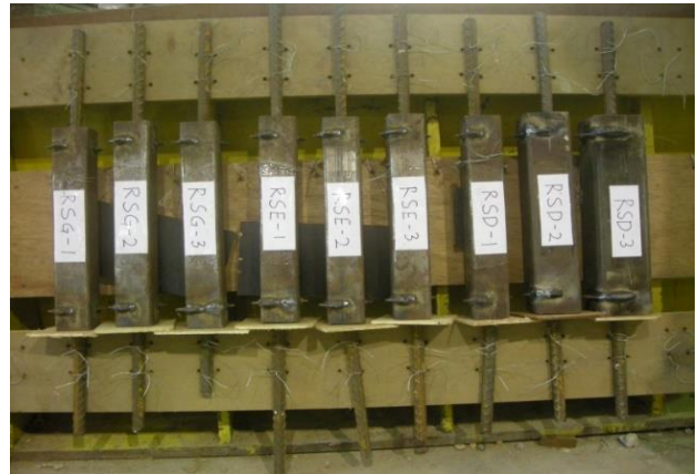
Figure 5 Pouring of Grout into Sleeves
