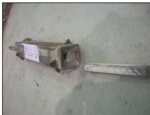
(a) Bar and grout failure
