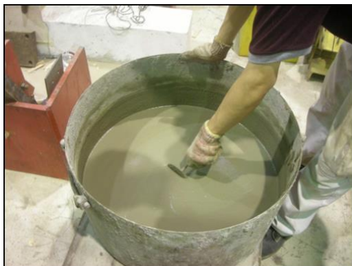
Figure 4 Preparation of grout
