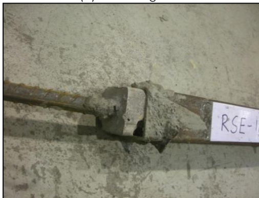
(b) Grout and sleeve failure
