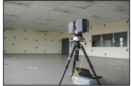
Figure 5 Self-calibration for the Faro Photo 120 scanner
