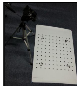
Figure 2 Photogrammetry self-calibration using Photomodeler V5.0 software
