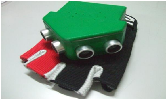
Figure 8 Final design/look of the sonar assistive device
