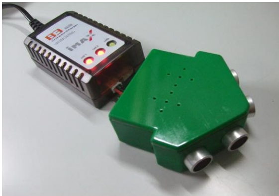
Figure 9 Charging of the device with the LIPO balance charger
