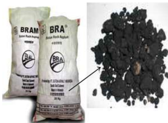
Figure 2 BRA in bag (left) and coarse grains of BRA (right) [8].
