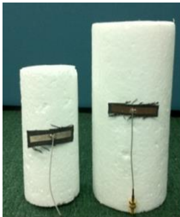
Figure 3 3.5cm and 7.0cm radius of Cylindrical Foams
