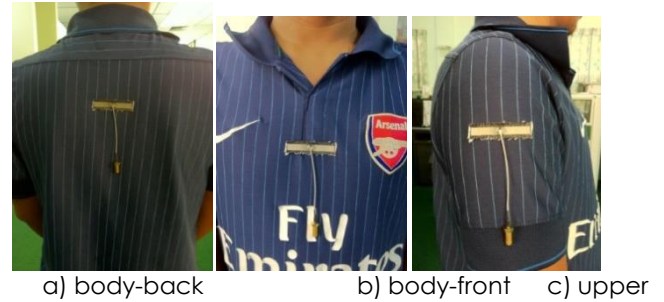
Figure 10 Locations of the Antenna on the human body measurement
