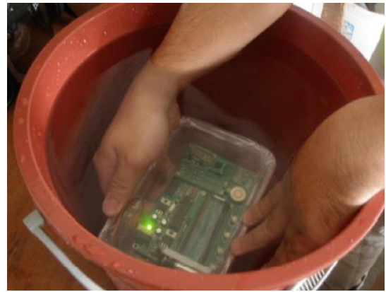
Figure 4(c) PR22 Board was Immersed in the tap water
