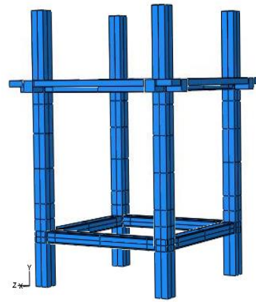
Figure 4 3D continuum brick element to model the frame using ABAQUS 6.8
