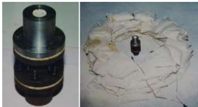
Figure 9 Full assembly of rocket motor (left) and ballistic test setup (right) 9
