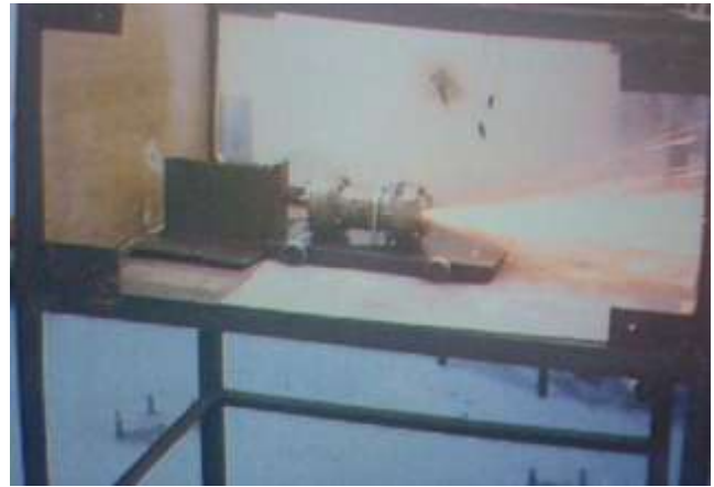
Figure 31 Potassium Nitrate based solid propellant in static test 30
