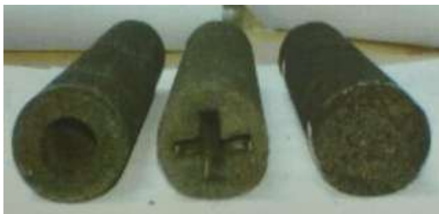
Figure 30 Grain configurations consist of tubular, star and end burner 29
