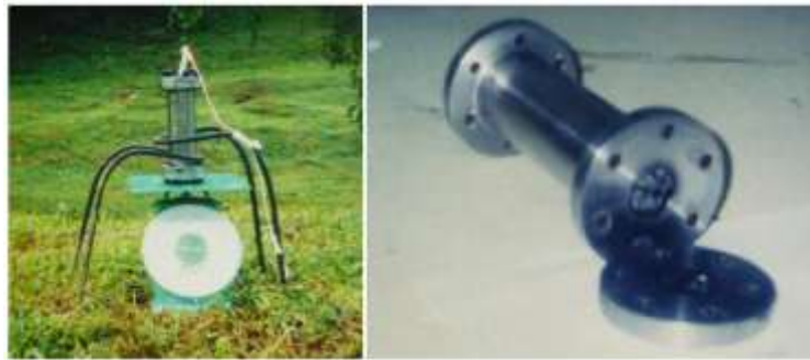
Figure 13 Simple thrust measurement apparatus with weighting machine (left) and rocket motor after firing test (right) 10
