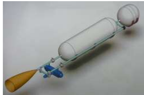
Figure 36 Conceptual design of hydrogen peroxide/kerosene liquid rocket engine 38
