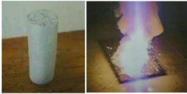
Figure 18 Grain sample with 25% lekar composition (left) and the propellant burning behavior under atmospheric pressure (right) 16
