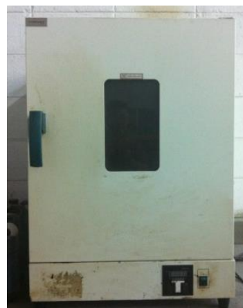
Figure 3 Forced draft oven
