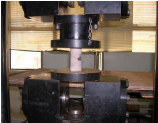
(a) UCS samples are ready to be tested
