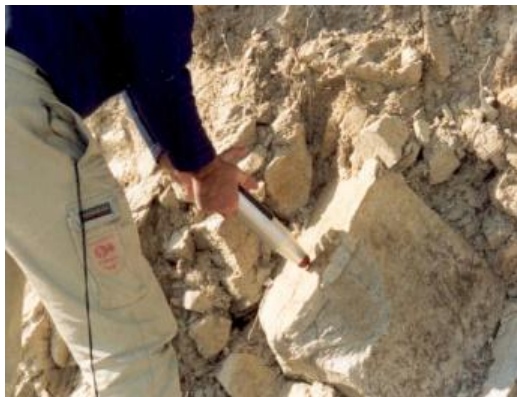
(c) Surface hardness test using rebound hammer
