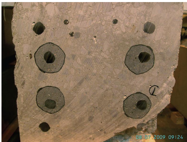
Figure 1.5 Cross section through grouted sleeve column splice [31]
