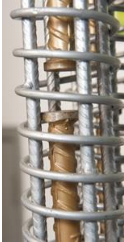
Figure 1.3 Spiral confinement in splice connections [29]
