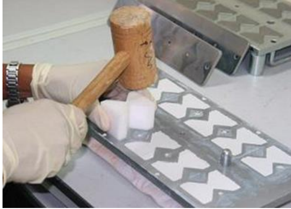
Figure 4 Specimen demoulding using Teflon block.
