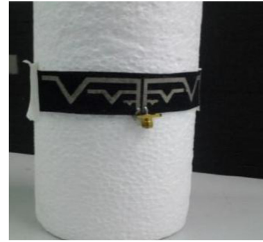
Figure 6. Koch fractal multiband antenna are bent on polystyrene cylinder.
