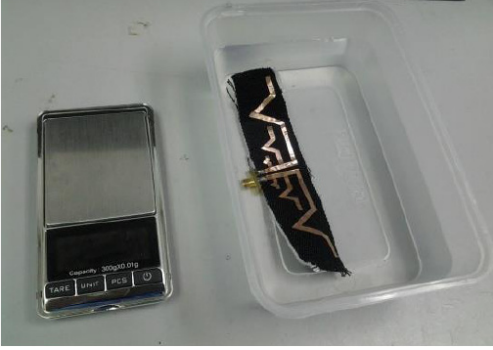
Figure 14. Fractal Koch multiband antenna are immersed in water.
